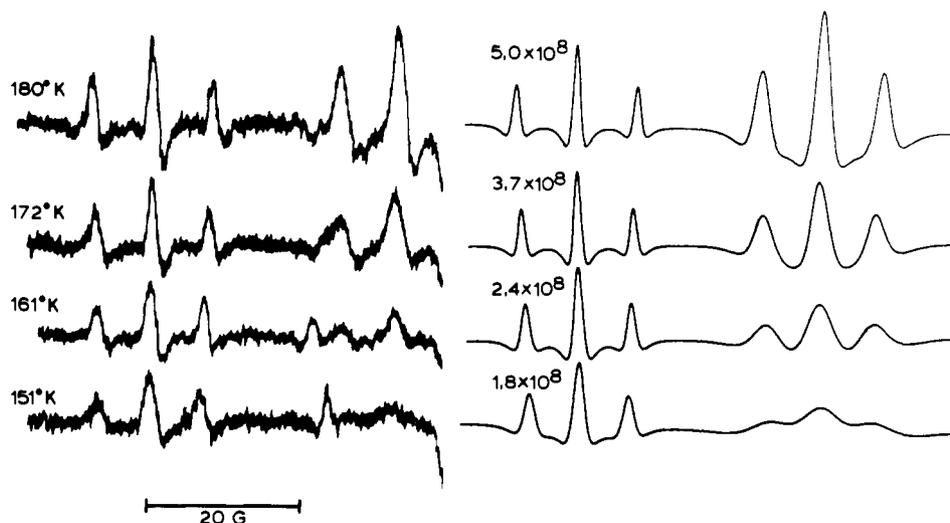
Figure 3. Expanded portion (see Figure 2) of the fluoromethylcyclopentyl radical spectrum as a function of temperature (left), with computer simulations (right). An impurity peak appears at lower temperatures.
