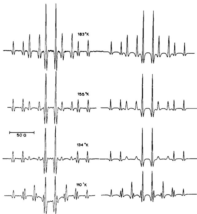
Figure 1. Second-derivative EPR spectra of the cyclopentyl radical in adamantane (left), with computer simulations (right).
