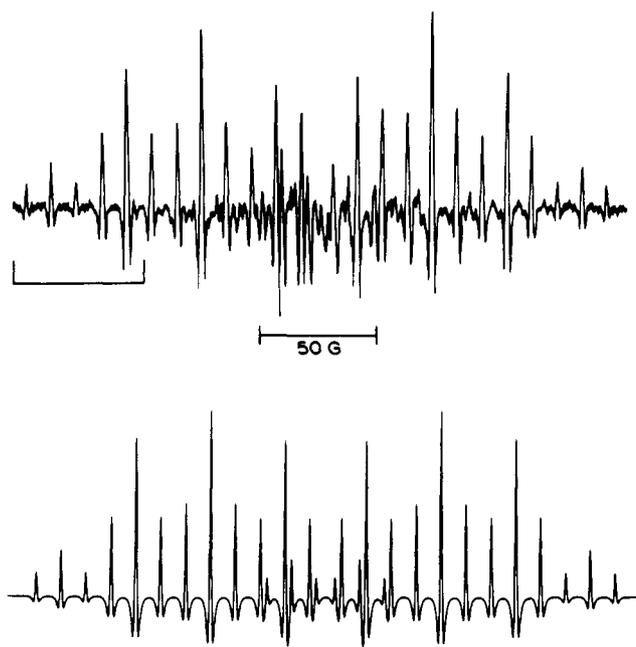
Figure 2. Second-derivative EPR spectrum of the fluoromethylcyclopentyl radical in adamantane- $d_{16}$  at 297 K (top), with a computer simulation (bottom). The lines shown in the bracket are expanded in Figure 3. There are several impurity peaks present in the center of the spectrum.
