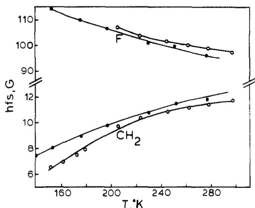
Figure 6. The temperature dependences of the fluorine and methylene proton hyperfine splittings in the fluoro-*tert*-butyl radical from ref 10 (closed circles) and the fluoromethylcyclopentyl radical (open circles). Note the change in the vertical scale.
