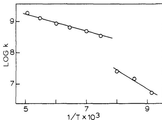
Figure 5. Arrhenius plot (see caption for Figure 4) for the cyclopentyl radical. The higher temperature line is the same as that shown in Figure 4.
