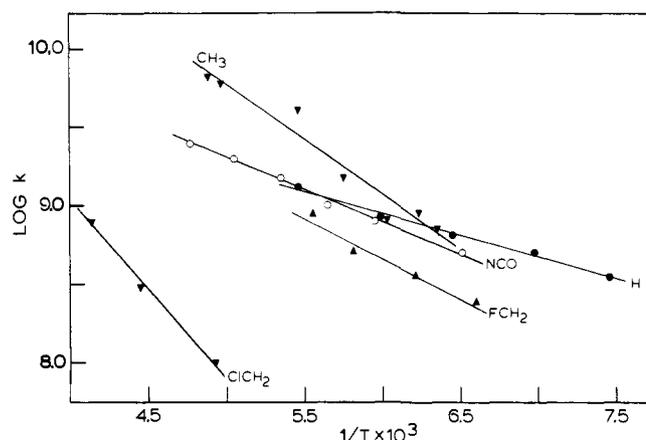
Figure 4. Arrhenius plots of the logarithm of the exchange rate from computer simulations vs. the reciprocal of the absolute temperature for each radical studied with the "best" least-squares straight line drawn through each set of points.
